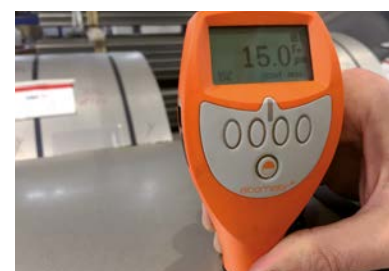
Coating thickness test Spessore rivestimento
