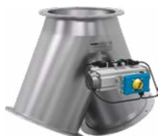
Example: Two-way valves with inner collar 50°, symmetrical, construction ND > 12" with welded-on flanges, pneumatically operated with a rotary actuator
